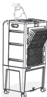
Refill water in the tank using tumbler from Ice box area
