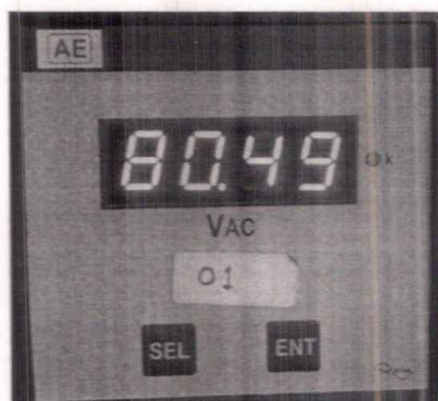
Setup for Low Voltage test (80VAC)
