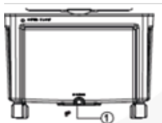
Remove the drain plug and drain all water out (Drain plug may be on the bottom side)
