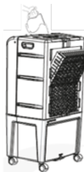
Refill water in the tank using tumbler from Ice box area (only in select models )
